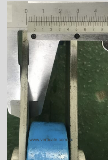
Chain Plate (Inner) 35mm (Height) x 5mm (Thickness)
